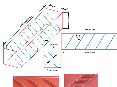
Fig. 2 The detail of inclined baffles
