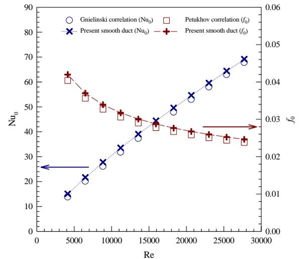
Figure 3. Validation of (a)  $Nu$  and (b)  $f$  for smooth duct.
